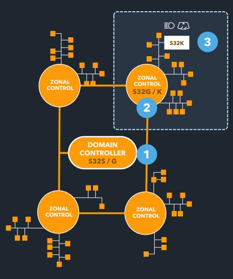
Ethernet bus routes communication from domains to physical zones of the vehicle
